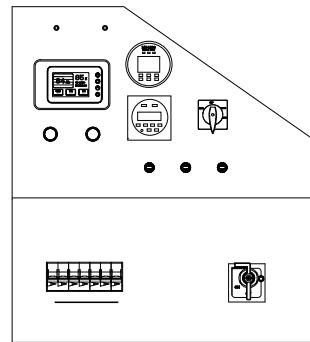
This control system is an advanced control module based on microprocessor, which is suitable for solar tower. The controller is equipped with a powerful graphical display that displays ICONS, symbols and bar charts for intuitive operation. Accurately measure various operating parameters, and display all values and alarm information on the LCD.
