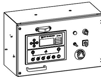
PLC-7420 is an advanced control module based on micro-processor, containing all necessary functions for protection of the genset and the breaker control. It can monitor the mains supply, and automatically start the engine when the mains is abnormal. Accurately measure various operational parameters and display all values and alarms information on the LCD. In addition, the control module can automatically shut down the engine and indicate the engine failure.
